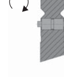
E2M®-HD Applicable for tool weight > 12.5 kg/28 lbs - < 100 kg/220 lbs (NS I & II)
