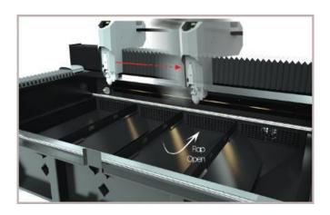
An automatic flap opens and closes according to the movement of the laser head, offering on-the-spot dust collection during cutting. This concentrates the vacuum in a single area for maximum efficiency.
