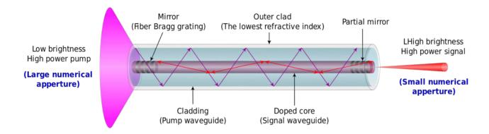
Inflated radiation is generated by a large number of laser diodes and is inputted into the optical fiber. There, with the help "Bragg mirrors", the wavelength of the generated laser beam is reduced to 1070  $\mu$ m. This wavelength is about one tenth of the wavelength of a CO<sub>2</sub> laser.
